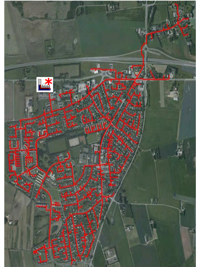
Harlev DHN which is used for simulation of its DHN in TERMIS
