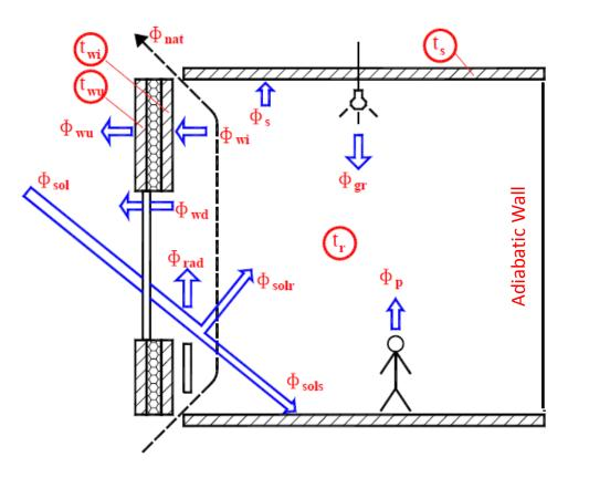
Lumped Capacity Model Technologies and S Based on SIMULINK dynamic model (MATLAB<sup>®</sup>)
