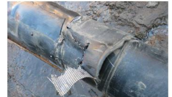
Fig. 4 - Shrink wrap peeled off due to the large number of movements.
