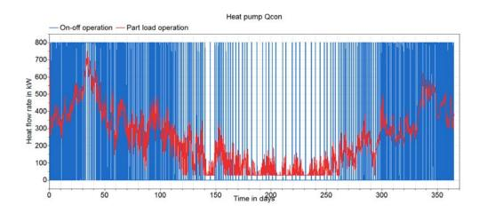
**On-Off operation** On-off according to storage state
